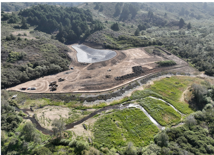
The Butano Creek Backfield Floodplain and Streamflow Enhancement Project completed in 2024, restored floodplain and riparian habitat, increased instream complexity, and supported farming by elevating the farm field and expanding a historical pond. See the pond in the background, the farm field in the middle, and the floodplain in the foreground.
