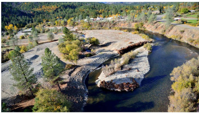
Apex bar jam redirecting flow into a side channel. Photo credit: David Bandrowski, Yurok Tribe.
