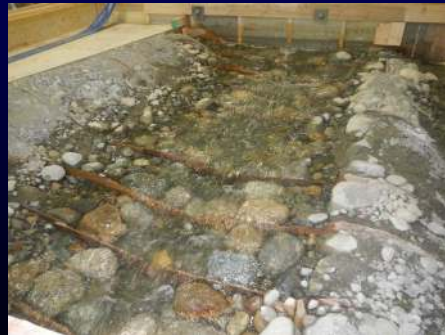
1:6 Model of Trabuco at Metrolink Cascade & Pool Roughened Channel
