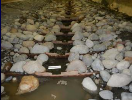
1:6 Model of Trabuco at Metrolink Cascade & Pool Roughened Channel
