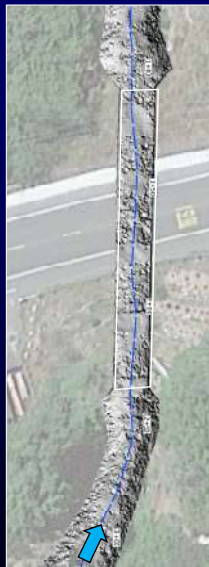
2D RAS Model built with Terrain from Scan of Bed
